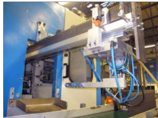
PHD Series SFP Slide installed on a Magic MP® extrusion blow moulding machine.
